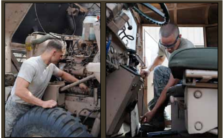
TSgt Adam Heath, 151st Logistic Readiness Squadron, examines a high-pressure oil line while working on an M-series wrecker at the Transit Center at Manas, Kyrgyzstan, July 26, 2011.
