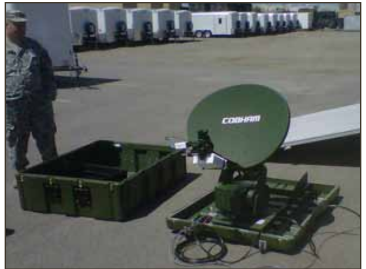
JOC Personnel test the new auto-acquire satellite dish after receiving it Aug. 15, 2011.
